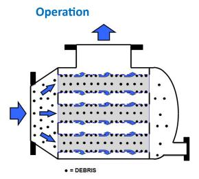
The raw liquid enters the filter baskets through the main inlet. The liquid is being filtrated when it passes through the filter—baskets prior to being discharged at the main outlet. The debris Is collected inside the baskets and in the debris collector. All loose debris collected can easaly be flushed out by opening the flushing valve installed at flushing outlet ( Can be ordered as extra).
